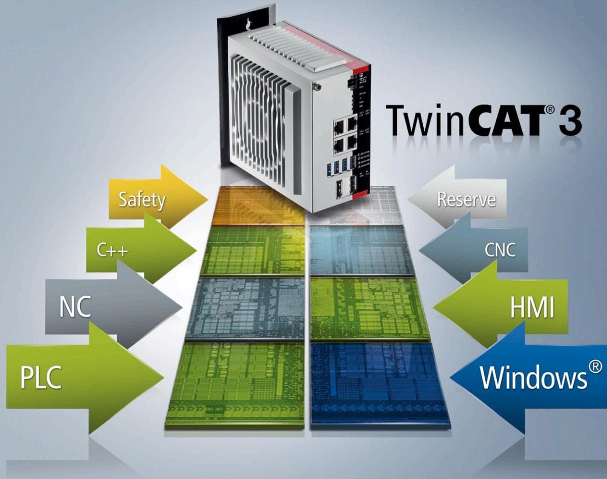
With the specially tailored TwinCAT 3 software and the increased granular scalability of its IPC products, Beckhoff makes the most of advanced multi-core technology. Shown here is the compact C6030 device with now up to eight processor cores.
